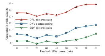
**Fig. 8.** This plots illustrates the sum of all capacities shown in Fig. 7. We see a clear increase in memory capacity as the feedback increases. The DRL post-processing scheme has the best capacity over the whole range, followed by the DNV post-processing scheme and lastly the conventional SNV post-processing.
