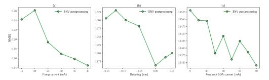
**Fig. 5.** The performance of the RC scheme as (a) the laser pump current is increased, (b) the wavelength detuning of the injected beam is varied and (c) as the sum of the current to SOA1 and SOA2 is increased. The performance is expressed by the normalized mean square error (*NMSE*). The results obtained here are from the single node value (SNV) post-processing scheme.
