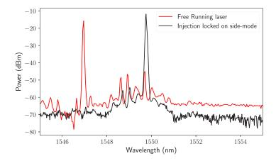
**Fig. 2.** The optical spectrum of the free running laser (red) superimposed on the spectrum of the injection locked laser (black). Injection locking was achieved at one of the side-modes at 1549.60 nm.
