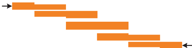
Fig. 5. The structure of the microstrip bandpass filter under study.
