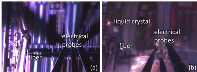
Fig. 7. Microscope image of the chip with fiber and electrical probes (a) before applying the liquid crystal, and (b) after applying the liquid crystal.
