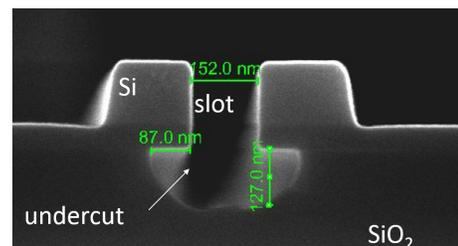
Fig. 5. SEM cross section of the slot waveguide after back-end opening.
