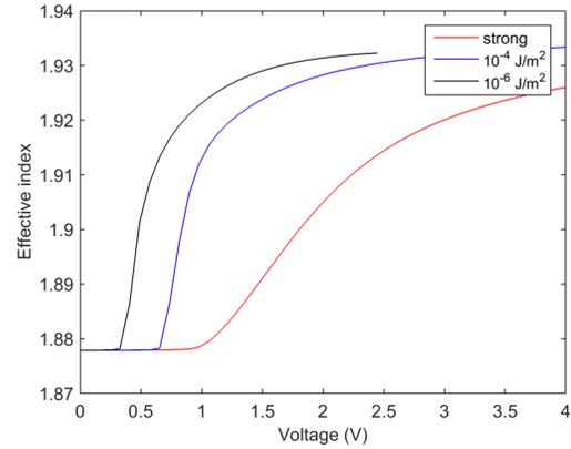
Fig. 4. Simulation of the effective index of the TE mode when applying a voltage over the liquid crystal in the slot waveguide, for different anchoring strengths of the silicon surface.
