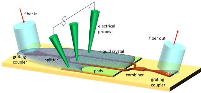
Fig. 6. Schematic of the measurement of the liquid crystal phase shifter. To characterize the phase modulator, the electrodes over one arm are shorted and grounded.
