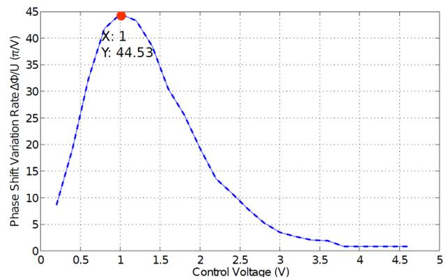
Fig. 9. Small signal modulation efficiency of a 1 mm long phase shifter as function of bias voltage. A maximum efficiency of  $44.53\pi/V$  is observed, corresponding to a modulation efficiency of  $V_{\pi} \cdot L_{\pi} = 0.0224V \cdot mm$
