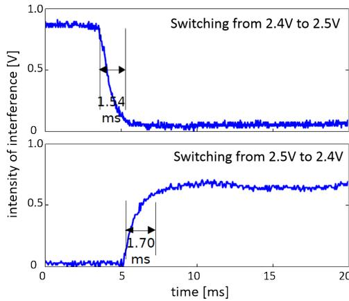
Fig. 10. Transient switch-on and switch-off transmission (Applying a  $\pi$  phase shift between a drive voltage of 2.4 V and 2.5 V)
