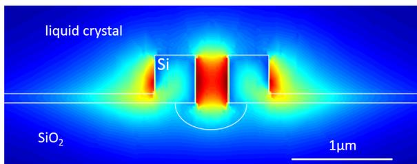
Fig. 3. Intensity profile of the TE mode in the slot waveguide without voltage.
