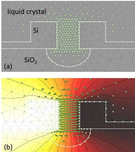
Fig. 2. Simulation of the E7 liquid crystal in the slot waveguides. The color background indicates the local electrical potential (a) Orientation of the LC molecules without bias, and (b) when a voltage is applied.
