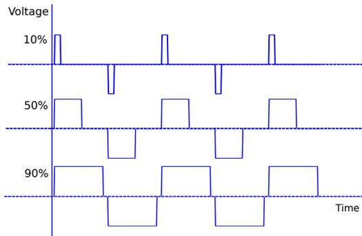
Fig. 11. Duobinary PWM drive signal.
