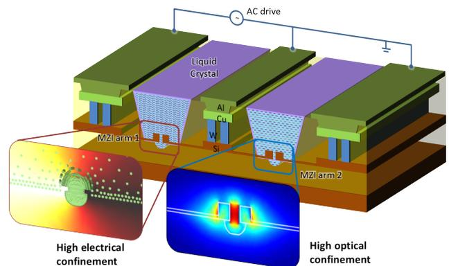
Fig. 1. Conceptual cross section drawing: The two arms of the Mach-Zehnder Interferometer have a slot waveguide infiltrated with liquid crystal.
