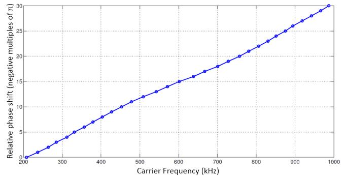
Fig. 13. Induced phase shift as a function of the AC frequency with constant amplitude of 1 V, relative to the shift at 200 kHz. Up to  $-30\pi$  phase shift can be obtained between 200 kHz and 1 MHz.
