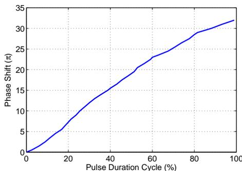
Fig. 12. Phase shift with increasing duty cycle of the PWM drive signal at 1.0V. We observe a phase shift of  $32\pi$ .
