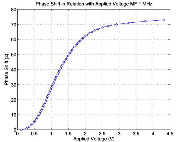
Fig. 8. Phase shift as a function of control voltage. A phase shift of  $73\pi$  is achieved at drive voltage of 5 V.
