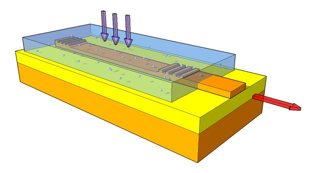
Figure: Simplified view of the laser structure.
