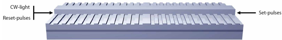
Fig. 2. Illustration of the concept for all-optical flip-flop operation.
