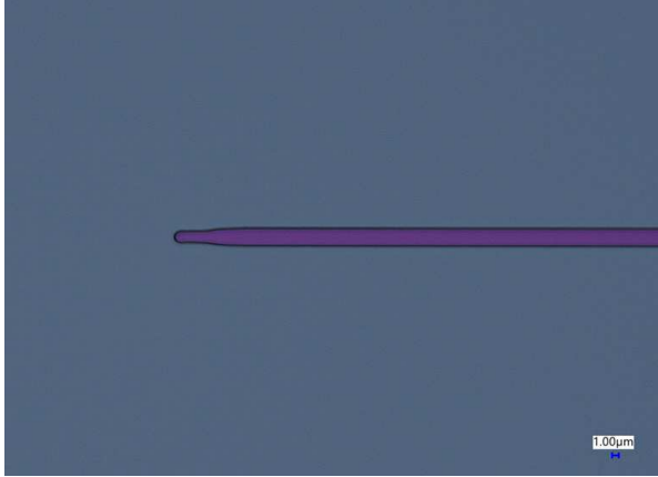
Figure 3.14: The mesa definition step using optical lithography. The mesa is defined by patterning the high resolution photoresist MIR-701 followed by the etching of SiNx
