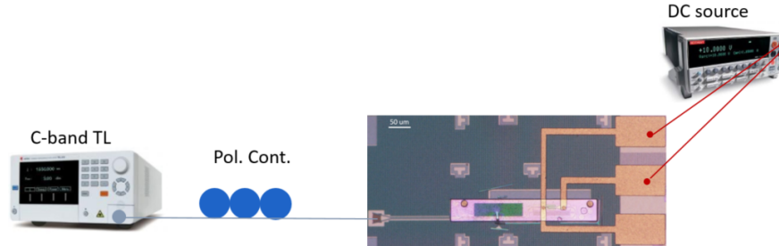
Figure 2.35: Responsivity measurement schematics.
