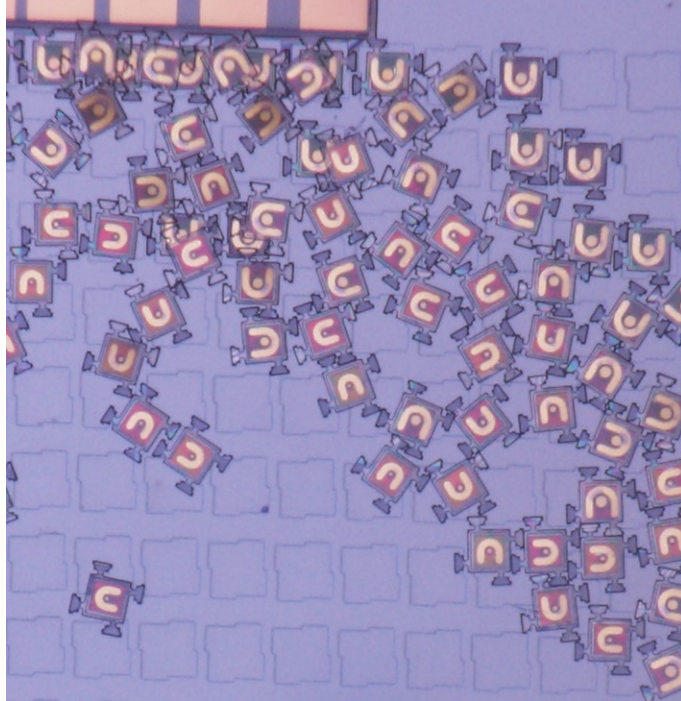
Figure 3.9: Example of bad adhesion of the photoresist tether to the source substrate.
