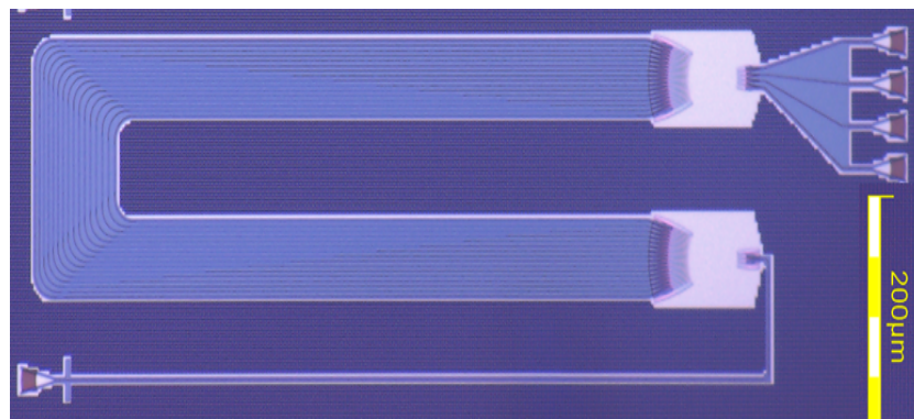
Figure 4.18: Fabricated all-silicon four channels athermal AWG
