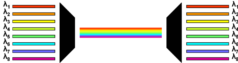
Figure 1.1: Scheme of an optical link utilizing wavelength-division multiplexing (WDM).
