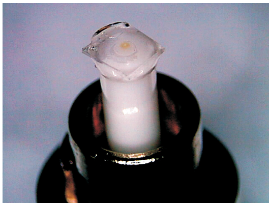
Figure 6.23: Microlens equipped SM fiber.
